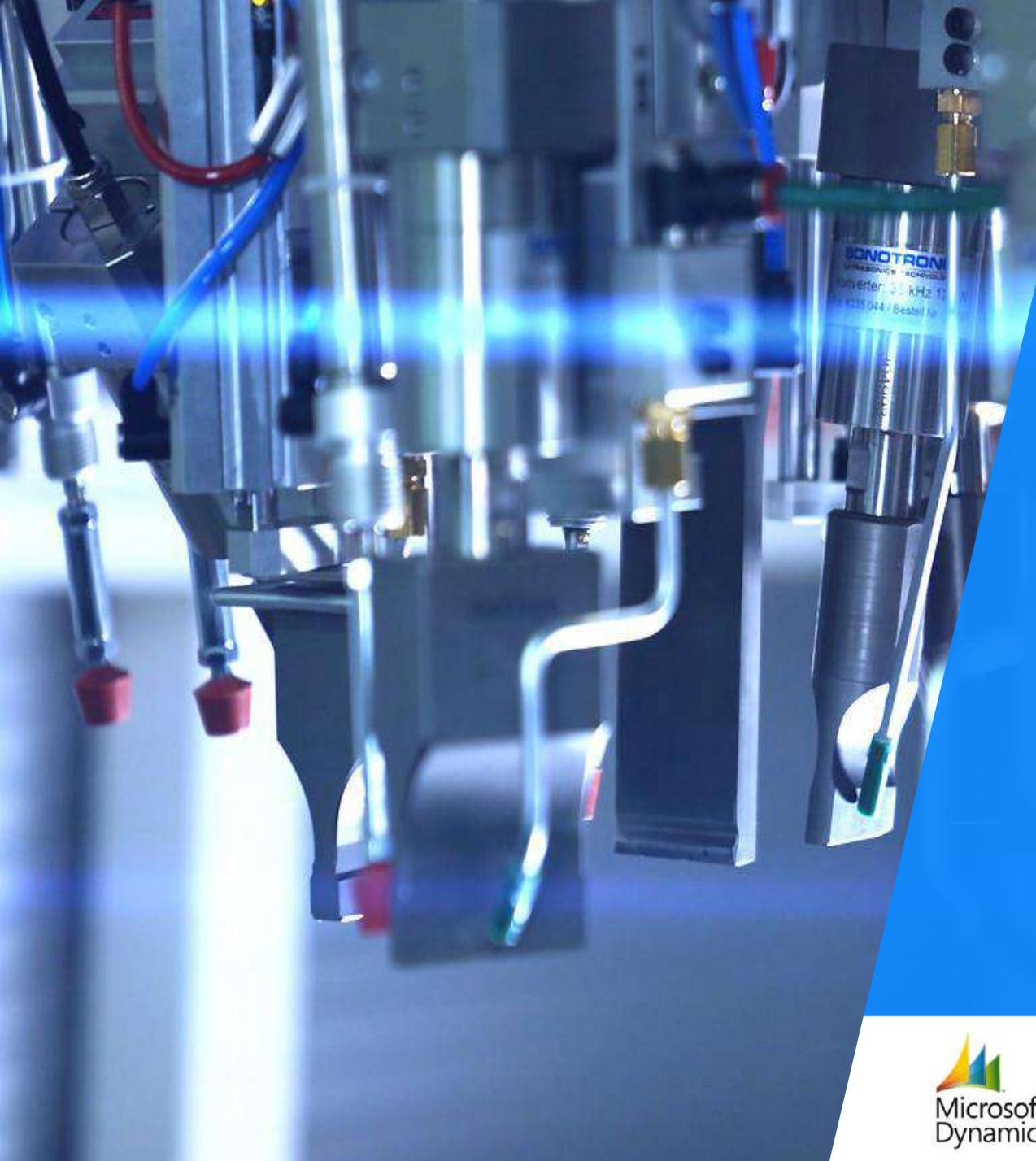
A close-up photograph of an industrial ultrasonic welding machine. The machine is primarily silver and black, with various cables (red, blue, black) connected to it. A prominent component is a vertical cylindrical ultrasonic converter, which has a label that reads "SONOTRONIC" and "Converter 35 kHz". The machine is set against a dark background, and the lighting highlights its metallic surfaces and the complexity of its assembly.
